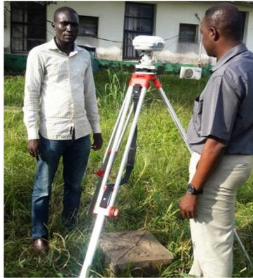
**Fig.3: Base Receiver at Control**
